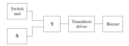
The alarm is triggered when a burglar stands on a pressure pad (the switch unit.). The buzzer then beeps on and off repeatedly.
