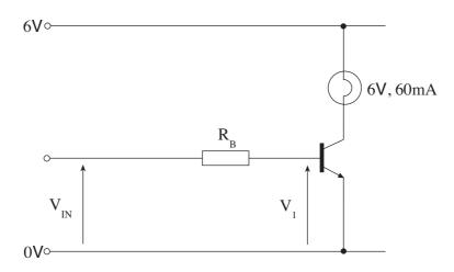
(a) The transistor is **just** saturated when the input voltage  $V_{IN}$  is 2.5V.
