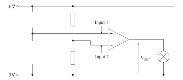
The output  $\boldsymbol{V}_{OUT}$  of the comparator saturates at +  $6\,\text{V}$  and  $0\,\text{V}$ *(a)*
