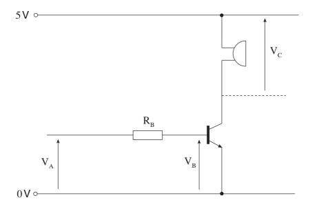
The transistor is just saturated when the input voltage  $\boldsymbol{V}_{\boldsymbol{A}}$  is  $2 \cdot 7 \, \textbf{V}.$
