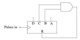
Complete the table to show the sequence of outputs produced, including the effect of the AND gate. [3]
