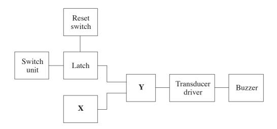
The alarm is triggered when a burglar stands on a pressure pad (the switch unit). The buzzer then beeps on and off repeatedly until the reset switch is pressed.
