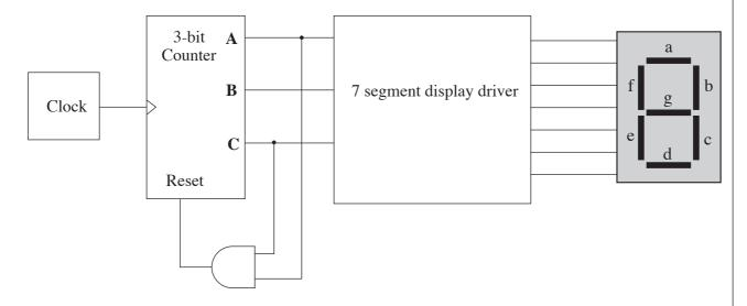
The counter is reset when it receives a logic 1 at the reset pin.
