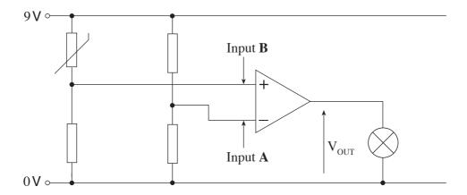
(i) The output  $\boldsymbol{V}_{\text{OUT}}$  of the comparator saturates at  $9\,\text{V}$  and  $0\,\text{V}.$
