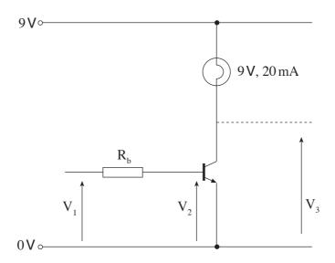
The transistor is just saturated when the input voltage  $\boldsymbol{V}_1$  is 2.7  $\boldsymbol{V}.$
