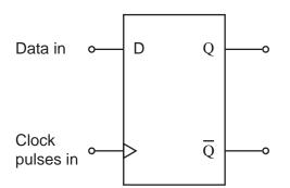
When the clock signal rises from logic 0 to logic 1: the Q output copies the logic level present on the clock input. the Q output copies the logic level present on the data input. the  $\overline{Q}$  output copies the logic level present on the clock input. the  $\overline{Q}$  output copies the logic level present on the data input.
