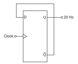
The Q output generates pulses with a frequency of 20 Hz.
