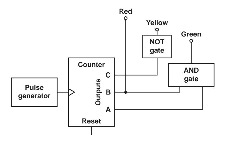
14. The diagram opposite shows part of a light sequence controller circuit, for three LEDs.
