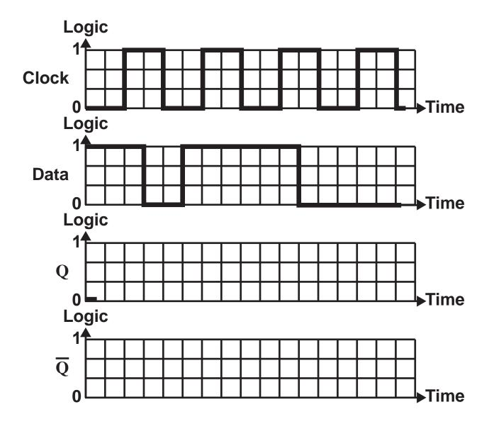
4(b) A rising-edge triggered D-type flip-flop receives the clock and data signals shown in the graphs opposite.
