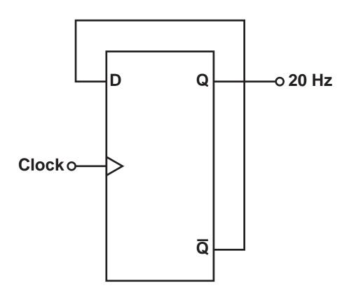
The Q output generates pulses with a frequency of 20 Hz.
