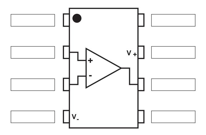
5. The diagram opposite shows the pinout of a comparator IC.
