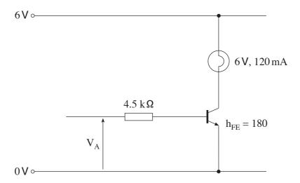
The transistor is just saturated.
