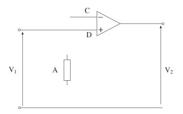
(i) Which input, C or D, on the diagram is the **inverting input**?
