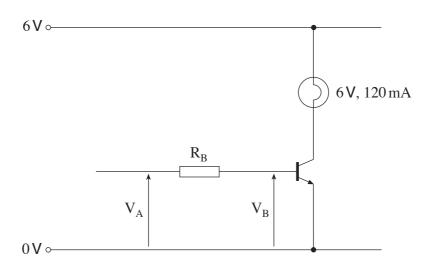
The transistor is **just** saturated when the input voltage  $V_A$  is 3.1 V.
