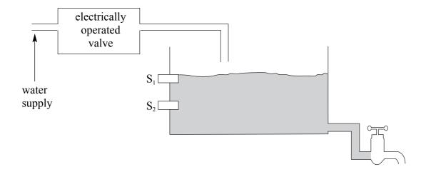
The signals generated by the sensors are different.  $S_1$  gives a high output when it is in water and a low output when it is dry.  $S_2$  gives a high output when it is dry and a low output when it is in water.
