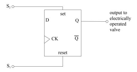
The valve opens when the Q output of the flip-flop is high.
