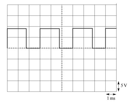
(i) The timebase is set to 1 ms per division. Use the oscilloscope trace to find the period of the pulses.
