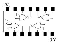
The network of gates is to be made on prototyping board. Complete the circuit below by adding the **five** wire links needed.
