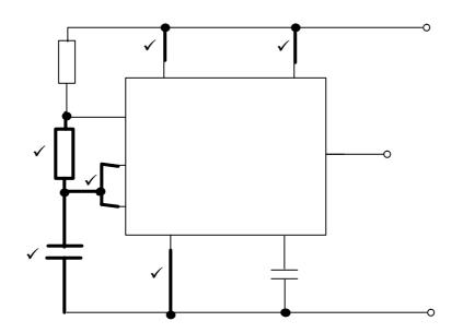
(b)  $T = (R_1 + 2R_2)C/1.44\checkmark = 31\checkmark s\checkmark$
