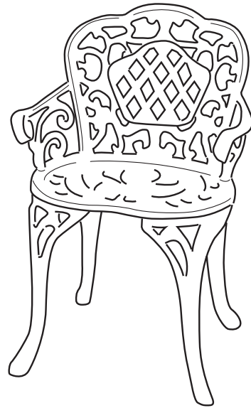
Chair B made from cast aluminium alloy
