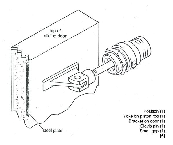
(b) When the piston stops moving forward, the pressure in the exhaust line and pilot line to the diaphragm valve reduces (1). When this happens the diaphragm will reset, by the spring (1) and causes a pilot signal to be sent to the 5/2 valve (1). This causes the direction of the air flow to the cylinder to be reversed (1) repressurising the pilot line which causes the valve to signal the piston to instroke (1).
