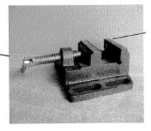
This is a small machine vice that's quite cheap. The threaded handle moves the jaw and a small screw in the jaw stops it from coming out when it is loosened
