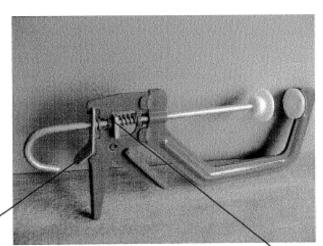
When the trigger is pulled this plate grips the shaft and pushes it forward
