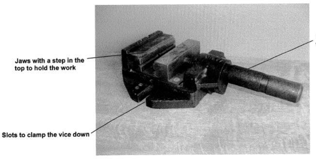
Handle with thread in to tighten and loosen the vice Most machine vices have got a screw thread in the handle to tighten the vice with and if you have a lot of pieces to drill it can take a long time to keep tightening and loosening the vice. It would be useful to have some sort of quick-release mechanism to tighten and loosen the vice so that lots of pieces that are the same could be drilled more quickly.
