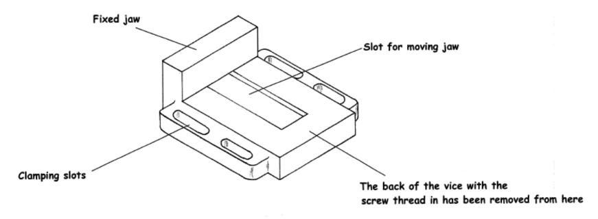
The base is made of cast iron because it is an awkward shape and because cast iron is heavy and slightly self-lubricating, so the moving parts can slide easily.
