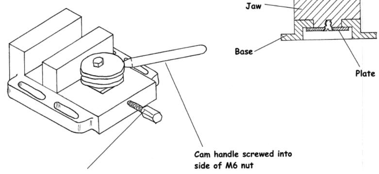
Adjustable stop to prevent cam support block moving back when the vice is tightened
