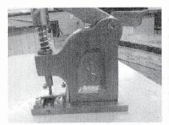
The metal work in my opinion is safe to use as it doesn't catch fingers or have any sharp edges, however because of the long handle it tilts forward when punched, but the back of the body casting is a perfect grip to solve this problem, or simply a vice mount could be added to solve this problem.
