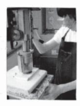
I started by culting a circular hole to fit a can in it. to cut this hole i used a hole sow on the pillar chill.
