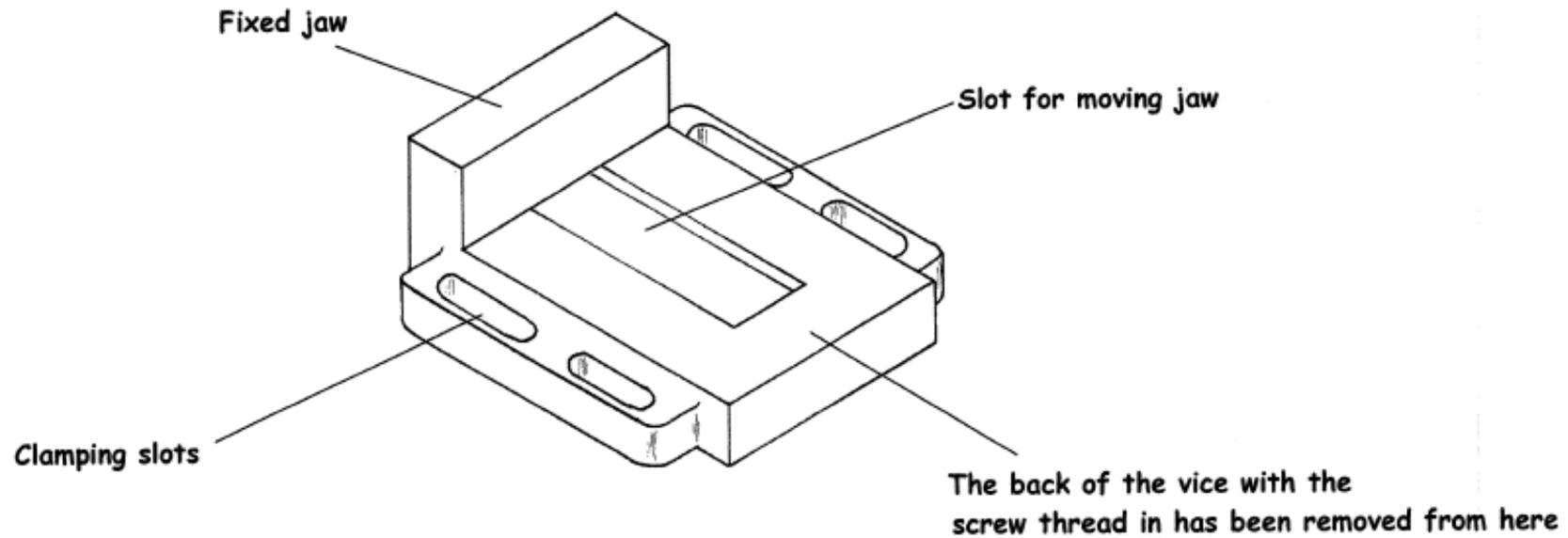
The base is made of cast iron because it is an awkward shape and because cast iron is heavy and slightly self-lubricating, so the moving parts can slide easily.
