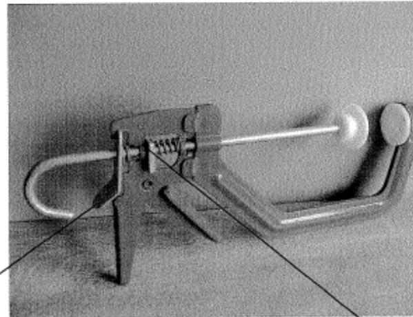
To loosen the clamp push this lever forward and pull the shaft back
