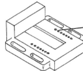
Tapped holes to fix block in place
