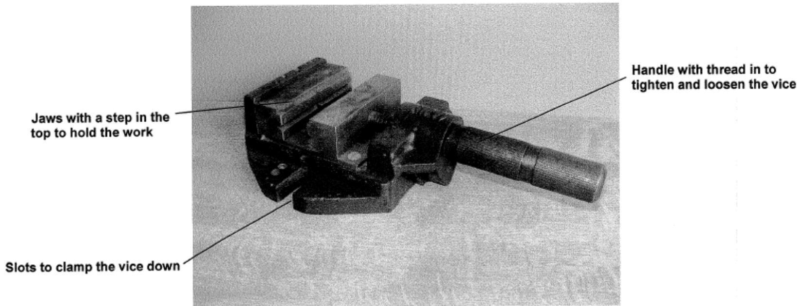
Most machine vices have got a screw thread in the handle to tighten the vice with and if you have a lot of pieces to drill it can take a long time to keep tightening and loosening the vice. It would be useful to have some sort of quick-release mechanism to tighten and loosen the vice so that lots of pieces that are the same could be drilled more quickly.
