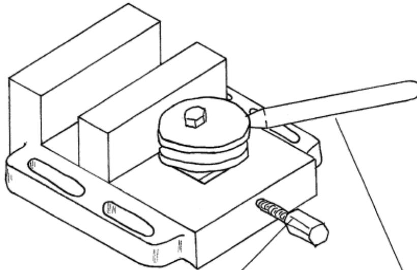
Adjustable stop to prevent cam support block moving back when the vice is tightened
