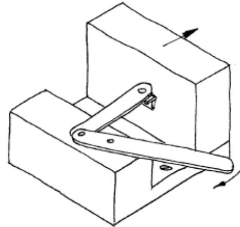
Lever used to move jaw backwards and forwards
