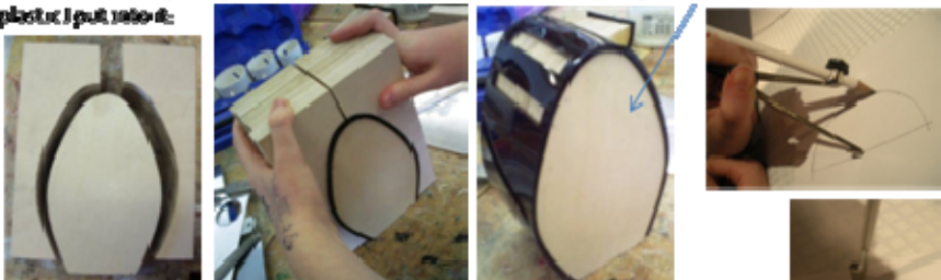
On the next slide, there are photos showing the continued process of how I made the St. Paul's mould and formed the plastic over it. The stages for making the moulds were the most time consuming, as I had to ensure they were the same sizes.
