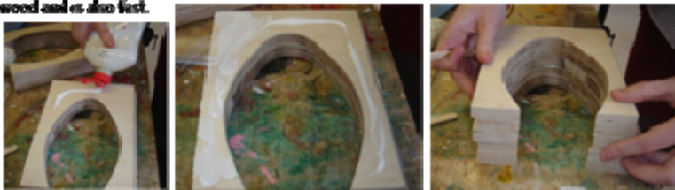
These pictures show the 'yoke' part of my mould for creating the curved surface of the Gherkin.
