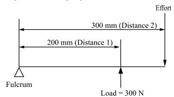
The load on the foot pump is 300 N.
