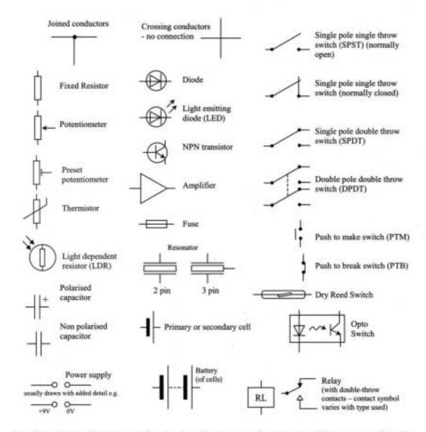
Note: Relay Symbol – The symbol consists of a relay coil and contacts. Contacts are usually drawn separate from the coil at convenient points on the circuit diagram and are always shown in the unoperated position.
