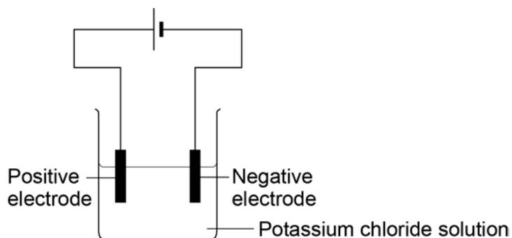
When the current is switched on, bubbles of hydrogen gas are given off at the negative electrode.
