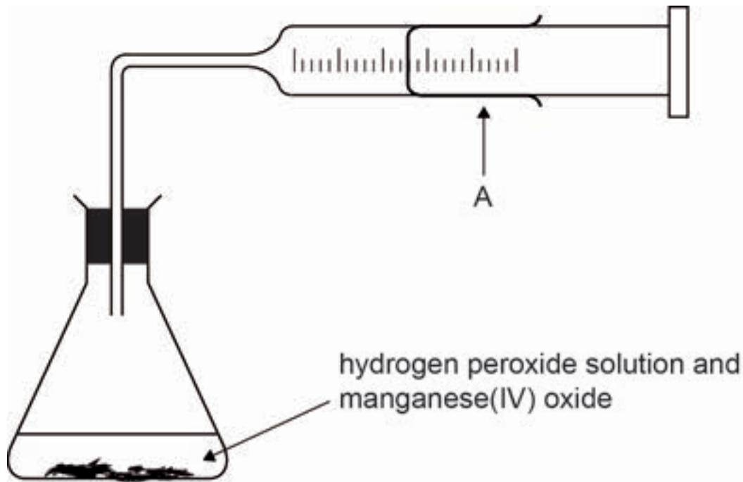
(i) Name the piece of apparatus labelled A. [1]
