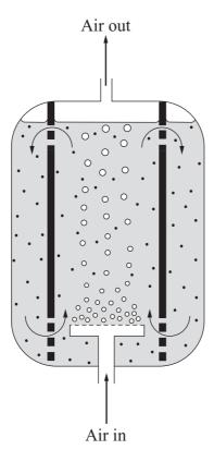
In this type of fermenter air is pumped in at the bottom.
