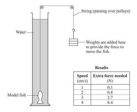
**10.1** The force needed to move the model fish . . . . .
