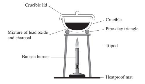
The mixture of lead ore and charcoal is heated in a crucible.
