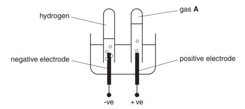
Hydrogen is made at the negative electrode.
