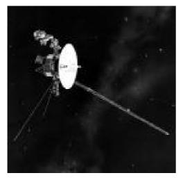
Voyager is so far away from Earth that a signal, travelling at the speed of light, takes over 12 hours to reach Voyager-1. By comparison, a signal sent to Mars, to command the Mars Global Surveyor spacecraft, takes only 15 minutes. The distance to the space craft can be calculated from the time taken for these signals to travel to the spacecraft.
