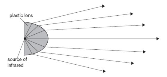
The LED is enclosed in a plastic lens.
