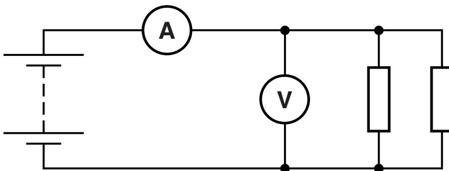
The diagram shows Alyson's circuit when she has TWO identical resistors in parallel.
