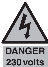
electrical shock hazard – 230 V
