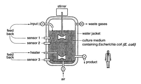
The fermenter has two separate feedback loops.
