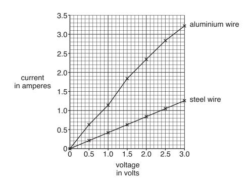
(ii) Use Miriam's results to calculate the conductance of the **steel** wire. Show your working.
