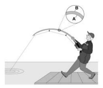
Which row in the table shows the type of stress that is acting at point **A** and at point **B** in the fishing rod?
