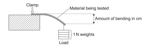
**7 (a)** Part of the material being tested is in compression. On the diagram, label the part in compression with the letter **C**.
