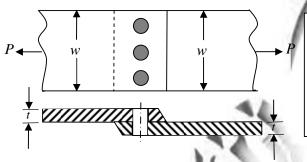
plate width w = 200 mmplate thickness t = 5 mmnumber of rivets n = 3rivet diameter  $d_r = 10 mm$ rivet hole diameter  $d_h = 11 mm$ allowable tensile stress of plate  $\sigma_p = 200 MPa$ allowable bearing stress of rivet  $\sigma_c = 150 MPa$
