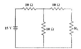
Assuming an ideal voltage source, Thevenin's resistance and Thevenin's voltage respectively for the above circuit are
