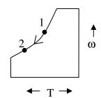
Since water content in moist air is reducing. The device is de-humidifier.
