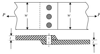
width of the plate w = 200 mm, thickness of the plate t = 5 mm, number of rivets n = 3, diameter of the rivet  $d_r = 10$  mm, diameter of the rivet hole  $d_h = 11$  mm, allowable tensile stress of the plate  $\sigma_p = 200$  MPa, allowable shear stress of the rivet  $\sigma_s = 100 MPa$  and allowable bearing stress of the rivet  $\sigma_c = 150 MPa$ .
