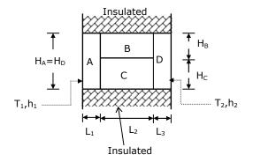
The dimensions are:  $H_A = H_D = 3m$ ,  $H_B = H_C = 1.5$  m,  $L_1 = L_3 = 0.05$ m,  $L_2 = 0.1$  m The thermal conductivity of the materials are:  $K_A = K_D = 50$  W/m-K,  $K_B = 10$ W/m-k,  $K_C = 1$  W/m-k.
