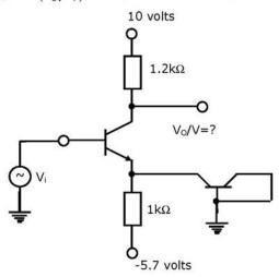
1.22. In figure the input  $V_1$  is a 100 Hz triangular wave having a peak to peamplitude of 2 volts and an average value of zero volts. Given that the diode is ideal, the average value of the output  $V_0$  is \_\_\_\_\_\_.
