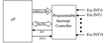
Assuming vectored interrupt, a correct sequence of operations when a single external interrupt (Ext INT1) is received will be :
