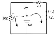
Steady state inductor behaves like short circuit
