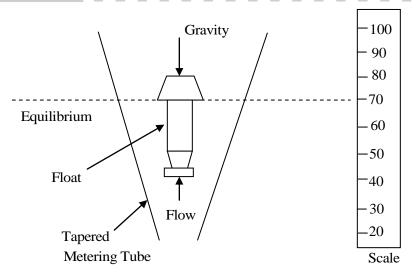
The flowing fluid enters the bottom of the meter, passes upward through a tapered metering tube, and around a float, exiting at the top. The float is forced upward until the force is balanced by gravitational force and drag force on float acting downwards.
