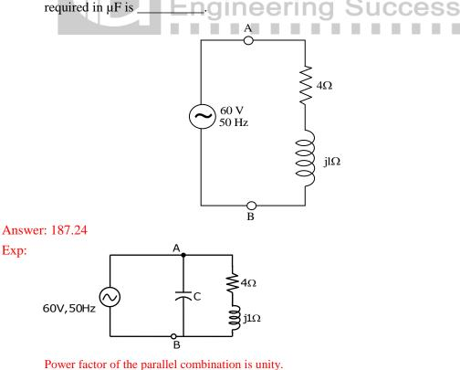
i.e., in total impedance equate the imaginary term to zero, which gives the capacitance required.
