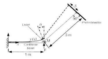
50. The translation S of the spot of laser on the photo-detector when a force of F=1N is applied to the cantilever is:
