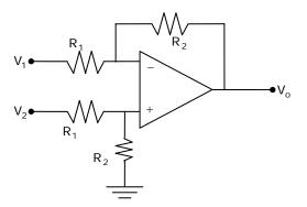
48. The input impedances seen looking into the terminals  $V_1$  and  $V_2$ , with respect to ground, respectively are
