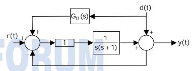
If the disturbance is measurable, its effect on the output can be minimized 57 significantly using a feedforward controller  $G_{f\ f}$  (s). To eliminate the component of the output due to  $d(t) = \sin t$ ,  $G_{f(jw)}|_{w=1}$  should be
