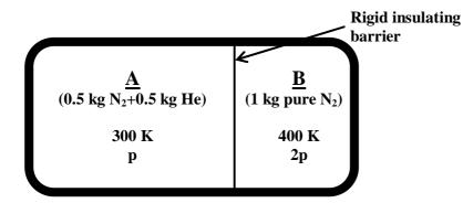
Specific Heat Data: For He  $c_p = 5181 \text{ J/kg.K}$  $c_v = 3102 \text{ J/kg.K}$ For N<sub>2</sub>  $c_p = 1039 \text{ J/kg.K}$  $c_{v}$ = 742 J/kg.K
