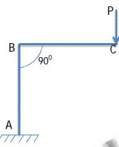
Neglecting the axial compression of member AB, the deflection of point C in the direction of the Q.17 load is
