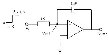
7. In figure, the operational amplifiers are ideal and their output can swing between -15 and +15 volts. Sketch on same diagram, the waveform of voltages  $V_1$  and  $V_2$  as a function of time. You must give the values of important parameters of this sketch.
