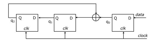
The following data: 100110000 is supplied to the "data" terminal in nine clock cycles. After that the values of  $q_2q_1q_0$  are:
