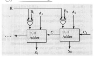
If the operands are in 2's complement representation, which of the following operations can be performed by suitably setting the control lines K and  $C_0$  only (+ and - denote addition and subtraction respectively)?
